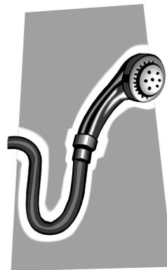
Hand-held shower heads which comply with state regulations for cross connection will have the code **ASME 112.18.1** stamped on the handle. In addition, make sure your hand-held shower head is at least 1 inch above the top of the flood level rim of the tub when it's hanging freely.
